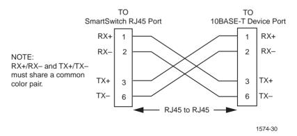
Figure 3-7 Cable Pinouts - (RJ45) Crossover Cable
